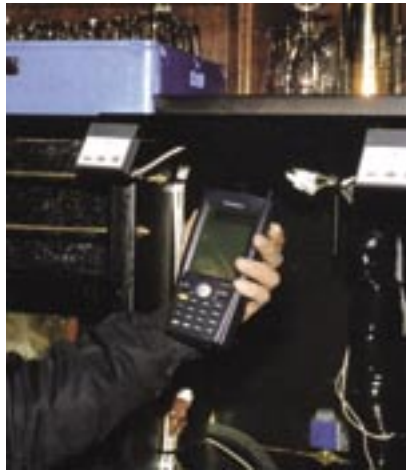
Service technician Øyvind Olsen scans the barcode on the beer tap to identify which equipment needs servicing.
